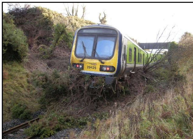
Photo 1 - Derailment in Co. Wicklow caused by third party works at the crest of a cutting.
